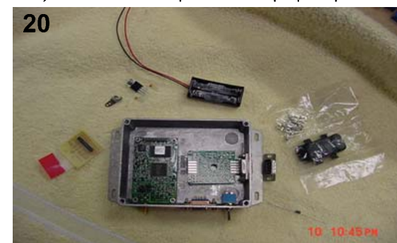
Install spacer hardware, mount GPS, TT3, Computer DB9, switch, and make any final adjustments. Locate, drill and mount the 7805 voltage regulator and the second ground lug (note ground lug on TT3 DB9). Remove all components and prep for paint.
