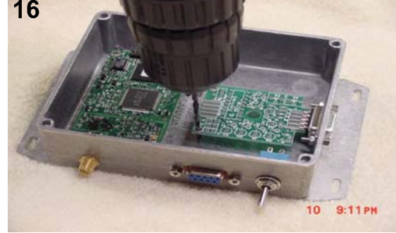
Countersink GPS and TT3 mounting holes (4)
