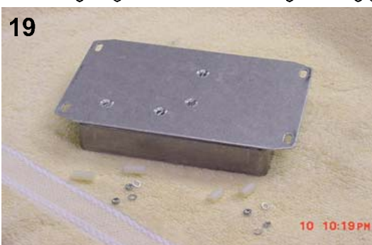
Install spacer hardware, mount GPS, TT3, Computer DB9, switch, and make any final adjustments. Locate, drill and mount the 7805 voltage regulator and the second ground lug (note ground lug on TT3 DB9). Remove all components and prep for paint.
