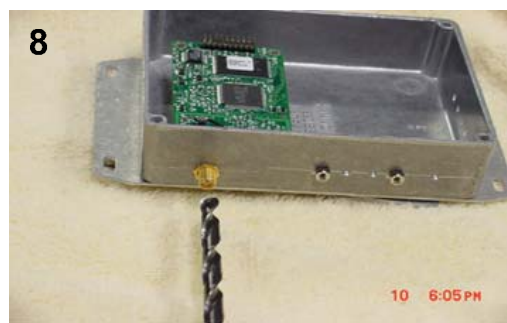
DB9 cutout, drill two .375 inch (or smaller) holes
