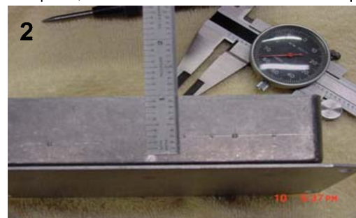
Computer, TT 3 and DPDT Sw 0.7 inch from top of box
