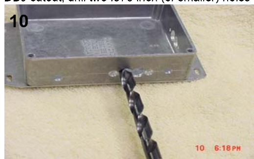
DB9 cutout, drill two .375 inch (or smaller) holes
